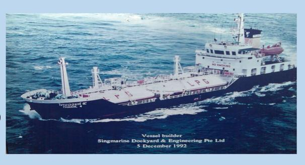
**Cargo Containment:** 2 Nos Cylindrical Tanks of 650 cbm at 18 kg/sq. cm pressure for carrying Propane, Butane or Propane / Butane mixture of any ratio.
