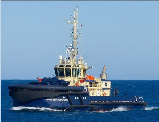
75T BP ASD HYBRID ESCORT TUG (for GORGON LNG project, Australia)
