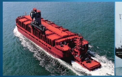
The barge is a covered deck-loading barge of 15,000 DWT equipped with self-unloader system supplied by BMH Marine AB, Sweden. A combined coal/oil barge equipped with BMH self-unloader system belongs to the fleet for supply of fuel to the mine and the loading site. The pusher boats, Tembaga 3 and 4, are powered with two Caterpillar 3606, each developing 2,300 KW at 1,000 RPM, to drive Schottel Rudder propellers SRP 2020.
