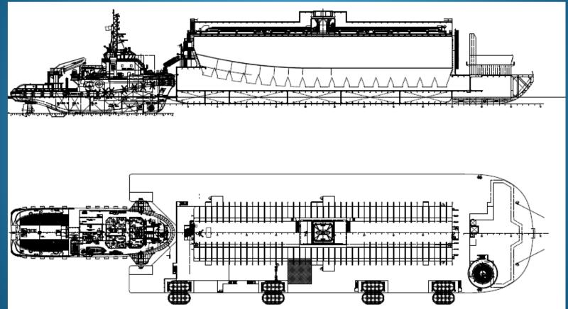
Scope of work includes design (incl stability check) and analysis (FEA) for sponson decks to house the articouple along with all necessary modifications for accommodating other equipment for Articouple system (such as HPU, accumulator unit, etc).
