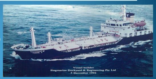
**Cargo Containment:** 2 Nos Cylindrical Tanks of 650 cbm at 18 kg/sq. cm pressure for carrying Propane, Butane or Propane / Butane mixture of any ratio.
